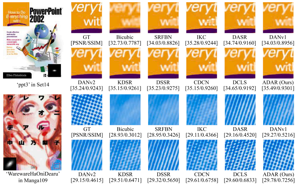
Fig. 10. Qualitative comparison of ADAR with other SOTA methods on \times 4 image SR of Set14 and Manga109 in Setting 2.
