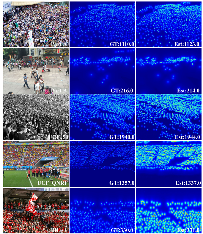
Fig. 5. Subjective results on crowd counting datasets. ‘GT’ and ‘Est’ indicate the ground truth and estimated value.
