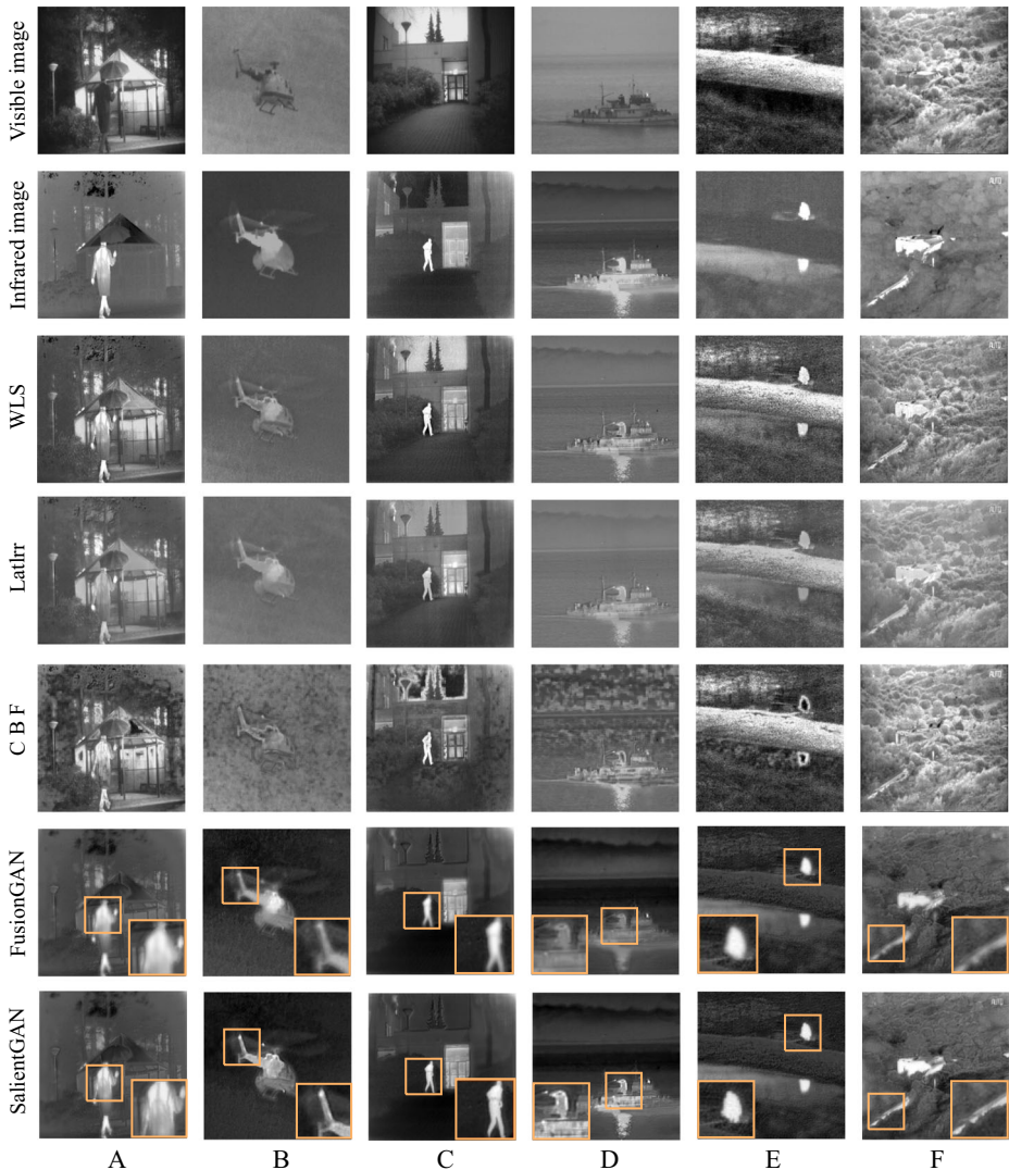
Fig. 6 Subjective comparison results on six representative IR and VIS image pairs from the TNO database [25]
