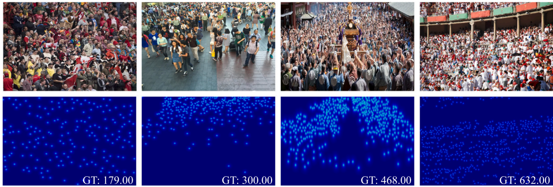
Fig. 1. Examples of congestion scenes in dense crowds. The first row is the input image, and the second row corresponds to the ground truth and the number of people.
